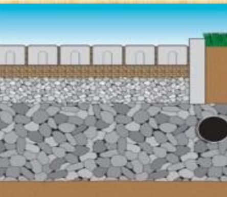
Pervious Pavement Source; www.greengaragedet.com/roit.com
